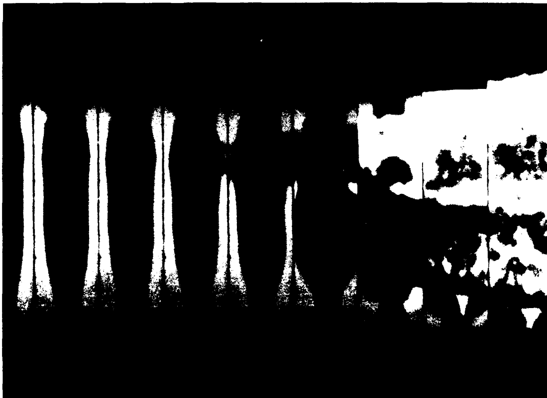
Figure 7: Print of a section of the camera record showing the expansion of a 105 mm shell undergoing a deflagration to detonation transition.
