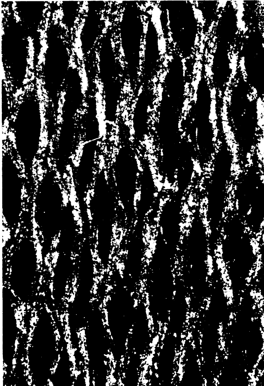
Figure 1 Microphotograph of Carbon/Carbon plate showing warp fibers
