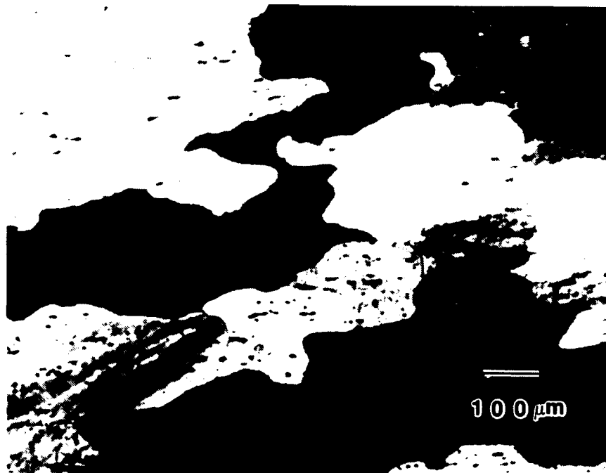
Figure 4.1 Al-Cu 2519 Alloy, After Overaging for 10 hours at 450°C. (a) SEM Backscattered Micrograph; (b) Optical Micrograph (x105).
