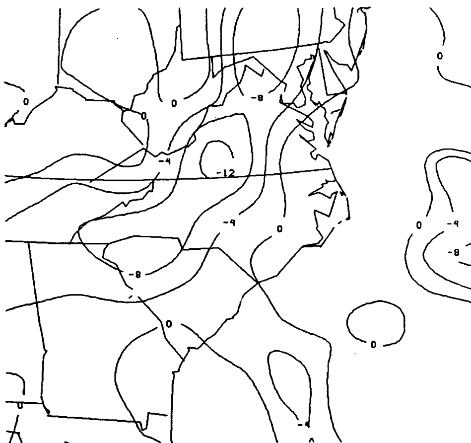
Fig. 7.2 Isopleths of the Laplacian of sea level pressure values for 1200 UTC, 25 January 1986. Values are given in units of \text{mb m}^{-2} .
