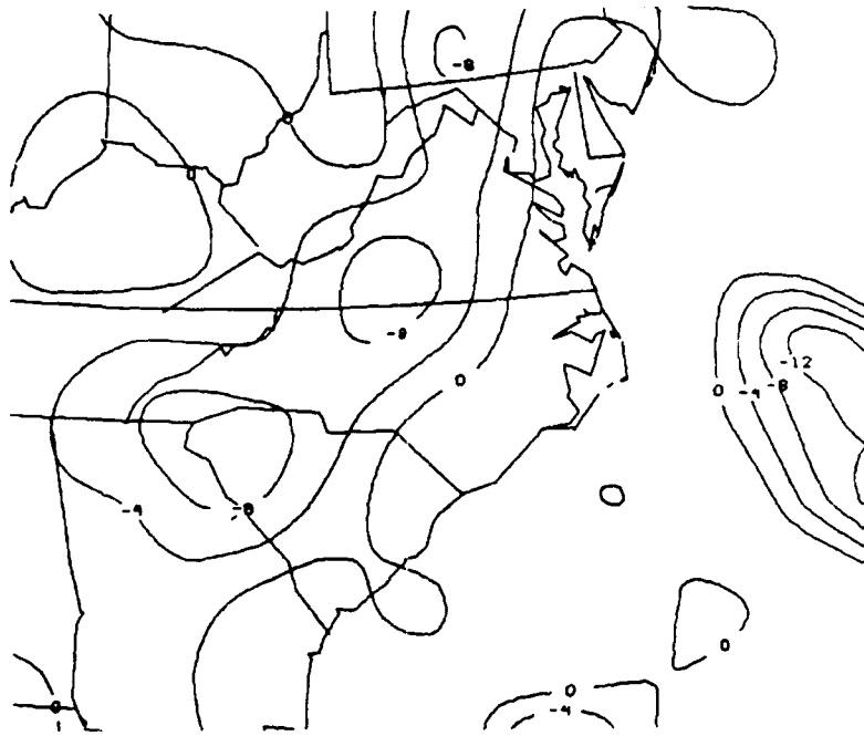
Fig. 12.15. Analysis of the Laplacian of sea level pressure valid at 1800 UTC 25 January 1986. Values given are \times 10^{-11} mb m^{-2} , and the contour interval is four units.
