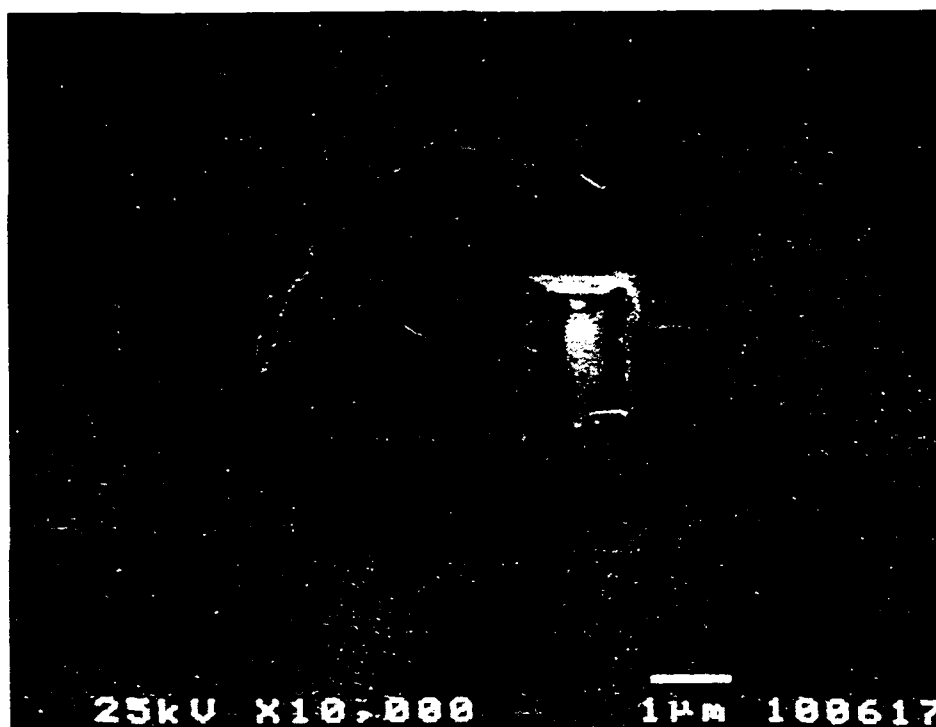
FIG. 4. Scanning electron micrograph of 0.3\text{-}\mu\text{m} -thick film grown in 10 hours from \text{CH}_3 + \text{H} on a diamond (100) substrate.
