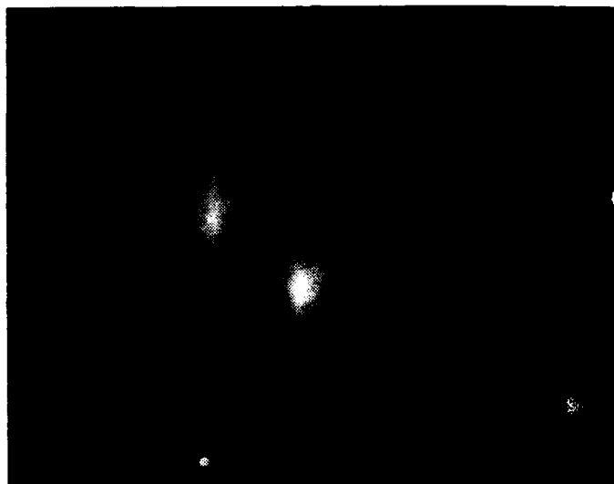
Figure 7. RHEED pattern produced upon exposure of diamond (100) surface to CO at 900°C. The weaker lines may be due to BCC iron.
