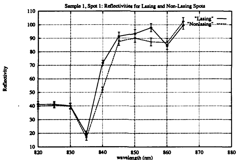
Figure 5.3. Sample 1 Measured Spectral Reflectivities for Lasing and Non-Lasing Locations near Spot 1
