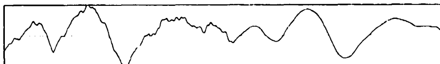
Figure 12. Advantage of a Smoothed EEG Signal. Note the multiple axis crossings in the original signal resulting from high energy, high frequency components. These crossings are absent in the smoothed version, leaving only the axis-crossings at the lower frequencies.
