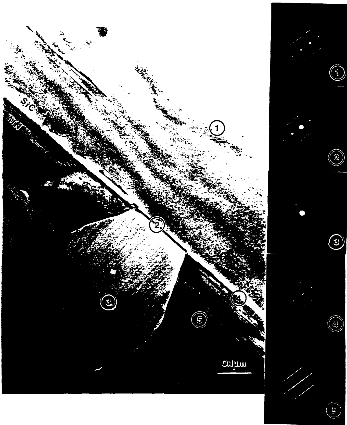
Figure 1. Cross-sectional TEM image of SiC-AlN at 1600°C for 200 hrs. and SAD patterns in several regions.
