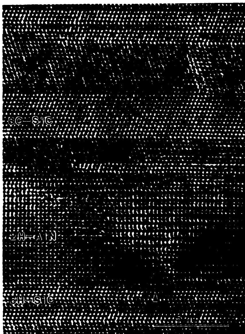
Figure 4. HRTEM micrograph of AlN film grown at 1050°C on vicinal 6H-SiC (0001). Layer above AlN layer is 3C-SiC also grown at 1050°C using gas-source MBE. Arrow points to dislocation in the AlN film at a step on the 6H-SiC surface.
