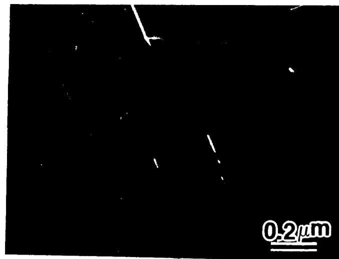
Fig.9 CDF image of plate-like precipitates formed from the pattern shown above
