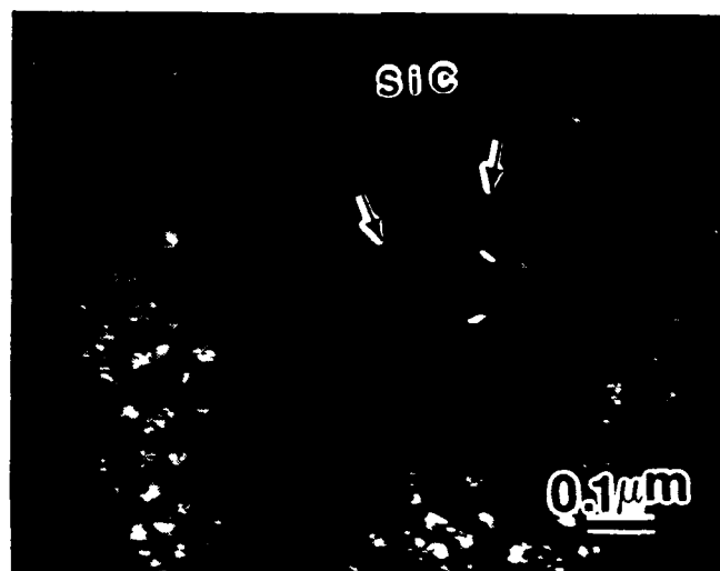
Fig.16(a) T2 (arrowed) phase at the SiC/matrix interface (25 hrs. of aging)
