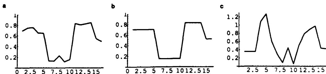
Figure 7.21: a) Input vector given to the trained feedforward network. b) Desired output of the network. c) Actual output of the network. This shows very poor generalization by the trained RBF network.
