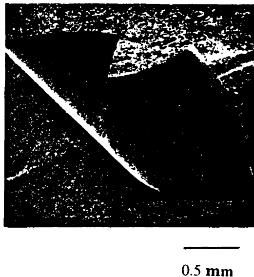
FIG. 3. Scanning electron micrograph of a lifted-off diamond layer. The liftoff was achieved by implantation with 5 MeV O ions to a fluence of 10^{18} \text{ cm}^{-2} , followed by annealing in flowing oxygen at 550 °C for 1 h. The sample was then vacuum annealed at 950 °C for 1 h to remove radiation damage.
