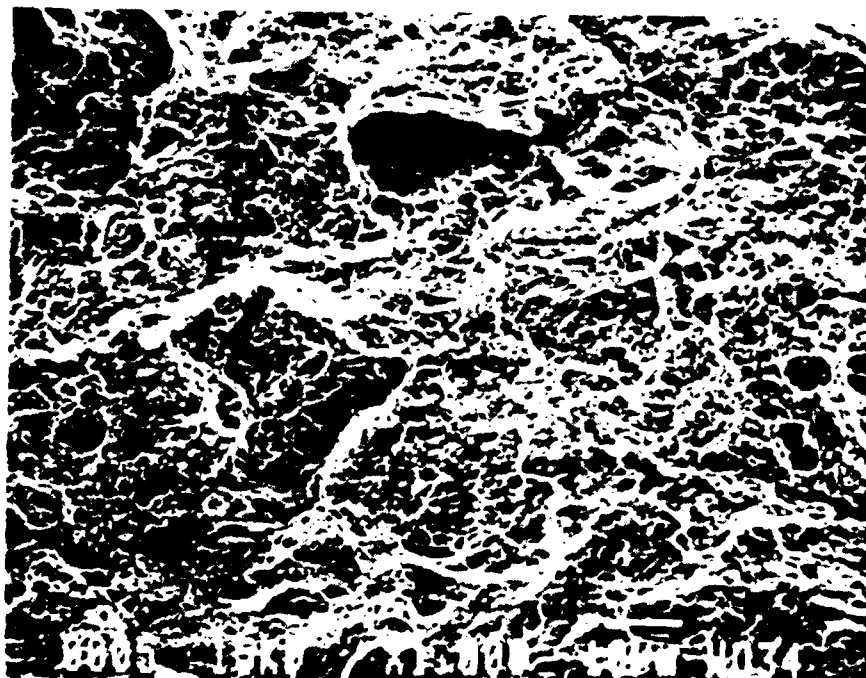
Figure 6. Scanning electron micrographs depicting the fracture surface morphology for Charpy specimen 2 machined from a pitch link retempered to HRC 38. This specimen had the lowest value in its lot, 33.0 ft-lb.
