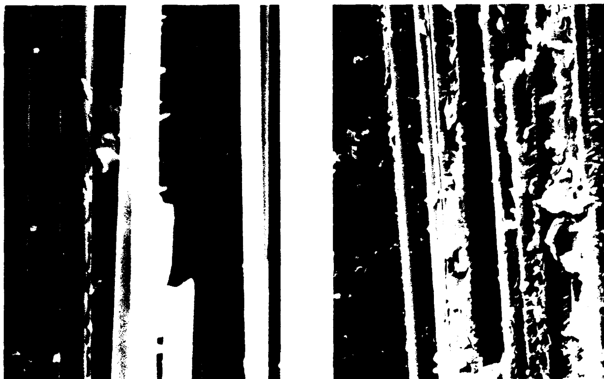
Figure 3. Evidence for poor interfacial adhesion in carbon/vinyl ester (left photo), showing low strength and bare fibers. The carbon/epoxy appears well-bonded (right photo) and has good properties.
