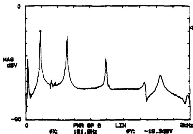
Fig.3: Frequency spectrum with no delamination
