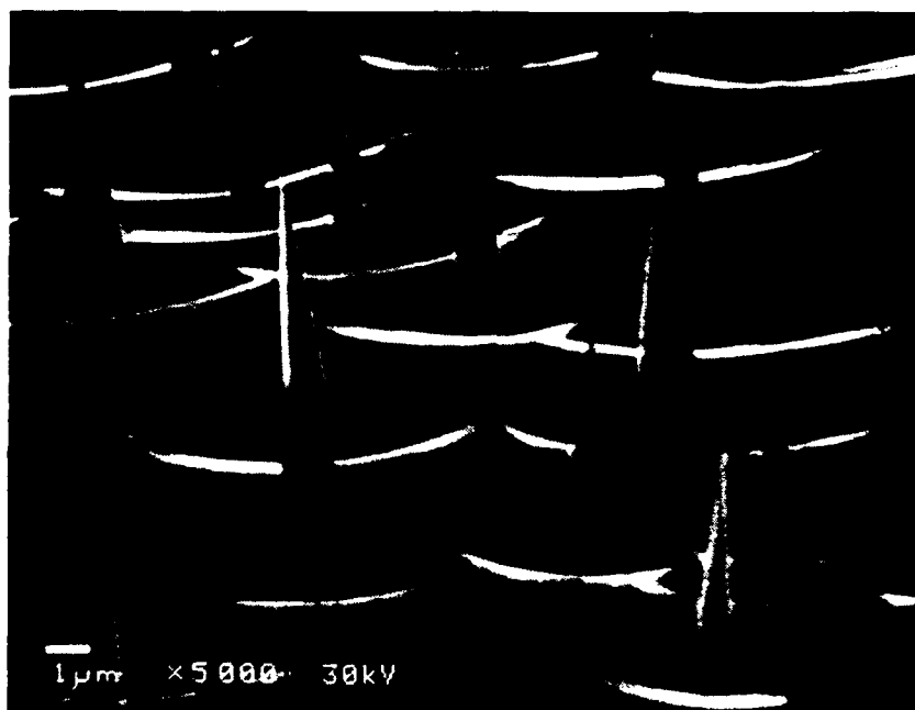
Figure 10. 7–8 \mu\text{m} height sharp-point \text{TaSi}_2 tips revealed by chemical etching.
