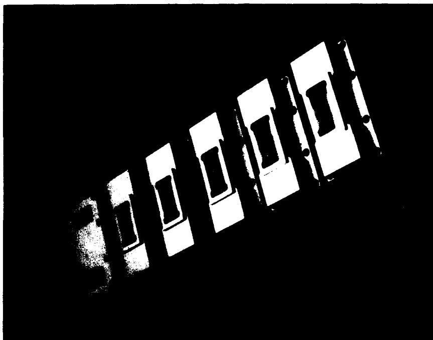
FIGURE 7. 55 Vol-% Al/SiC Driver Modules PCD-Machined From Forge-Clad Bulk Material.
