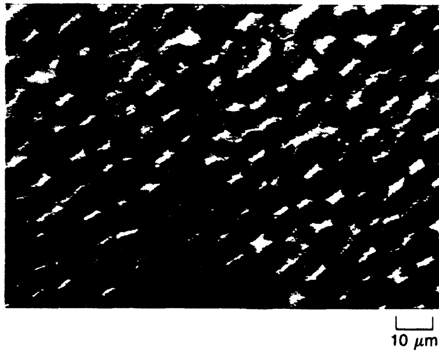
Figure 4. Scanning electron micrograph (SEM) of T-50/PAA-derived C/C composite heat-treated to 1100°C.
