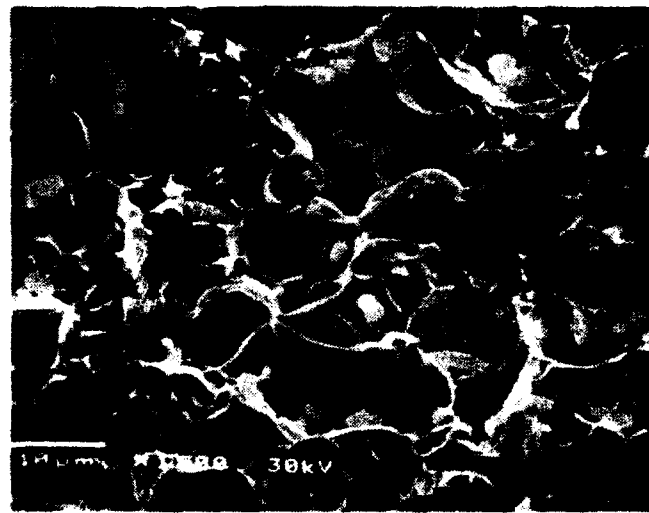
Figure 5. Fractographs of (a) \text{W}+7\% \text{Ni}_3\text{Al} (b) \text{W}+7\% \text{Ni}_{48}\text{Al}_{12}\text{Fe}_{40} .
