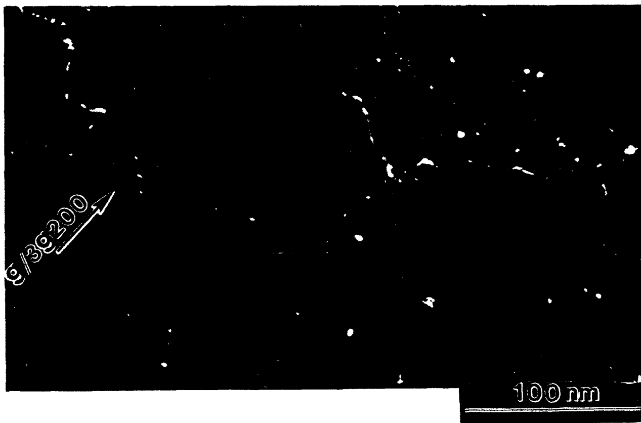
FIGURE 4. Dark field TEM images of the interior of a W grain: (A) two-beam image that shows the \sim 3.5 nm diameter precipitates to have black/white lobe contrast and (B) weak beam image of the same area that shows the precipitate strain contrast to be light on a dark background.
