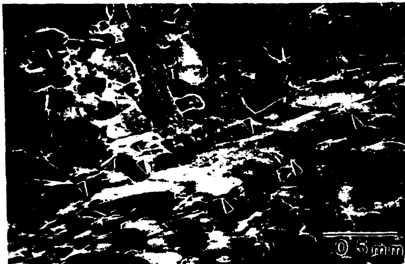
Figure 6. Optical micrograph of an as-deformed cross sectioned sample exhibiting localized flow instability within deformed pancake-shaped grains; see arrows.
