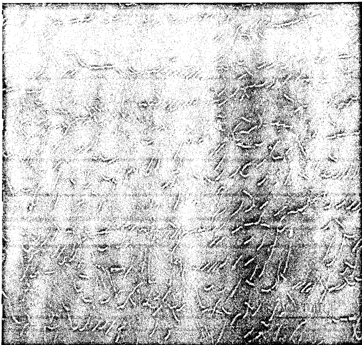
Fig.6 Dislocations in n-type GaAs grown by the horizontal Bridgman technique, as revealed by NIR transmission microscopy. (Compare with dislocation network in LEC GaAs.)
