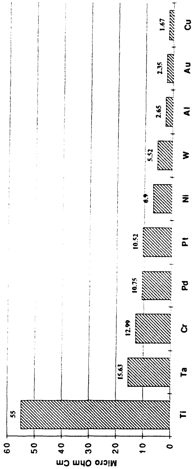
Figure B-4 ELECTRICAL RESISTIVITY OF SELECTED MCM METALS
