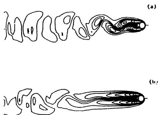
Figure 11: Downstream development of vorticity. a) natural shedding, b) suppressed shedding ( \alpha = 1.1 , x_s = -8 ).
