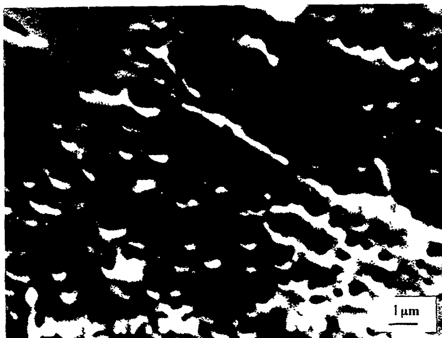
FIGURE 7.17(b) Scanning electron micrograph of an epoxy-film adhesive fracture surface (cohesive region). The joint was aged in the hot-wet environment for one year and then tested under static conditions. The substrate was U/C epoxy. Magnification X7,500.
