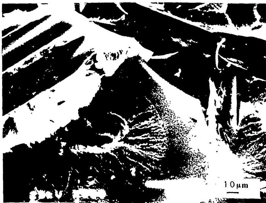
FIGURE 7.17(a) Scanning electron micrograph of an epoxy-film adhesive fracture surface (cohesive region). The joint was aged in the hot-wet environment for one year and then tested under static conditions. The substrate was U/C epoxy. Magnification X500.
