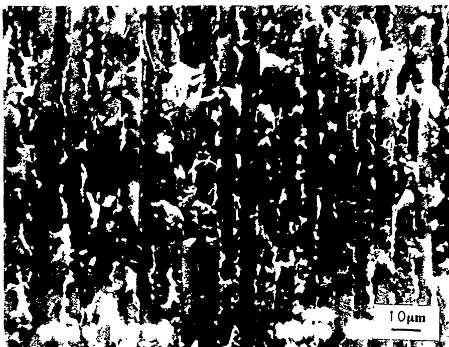
FIGURE 7.19(b) Scanning electron micrograph of the composite part of an interfacial fracture surface between the U/C PEEK composite and the epoxy-film adhesive. The joint was aged in the hot-wet environment for six months and was tested under static conditions. Magnification X750.
