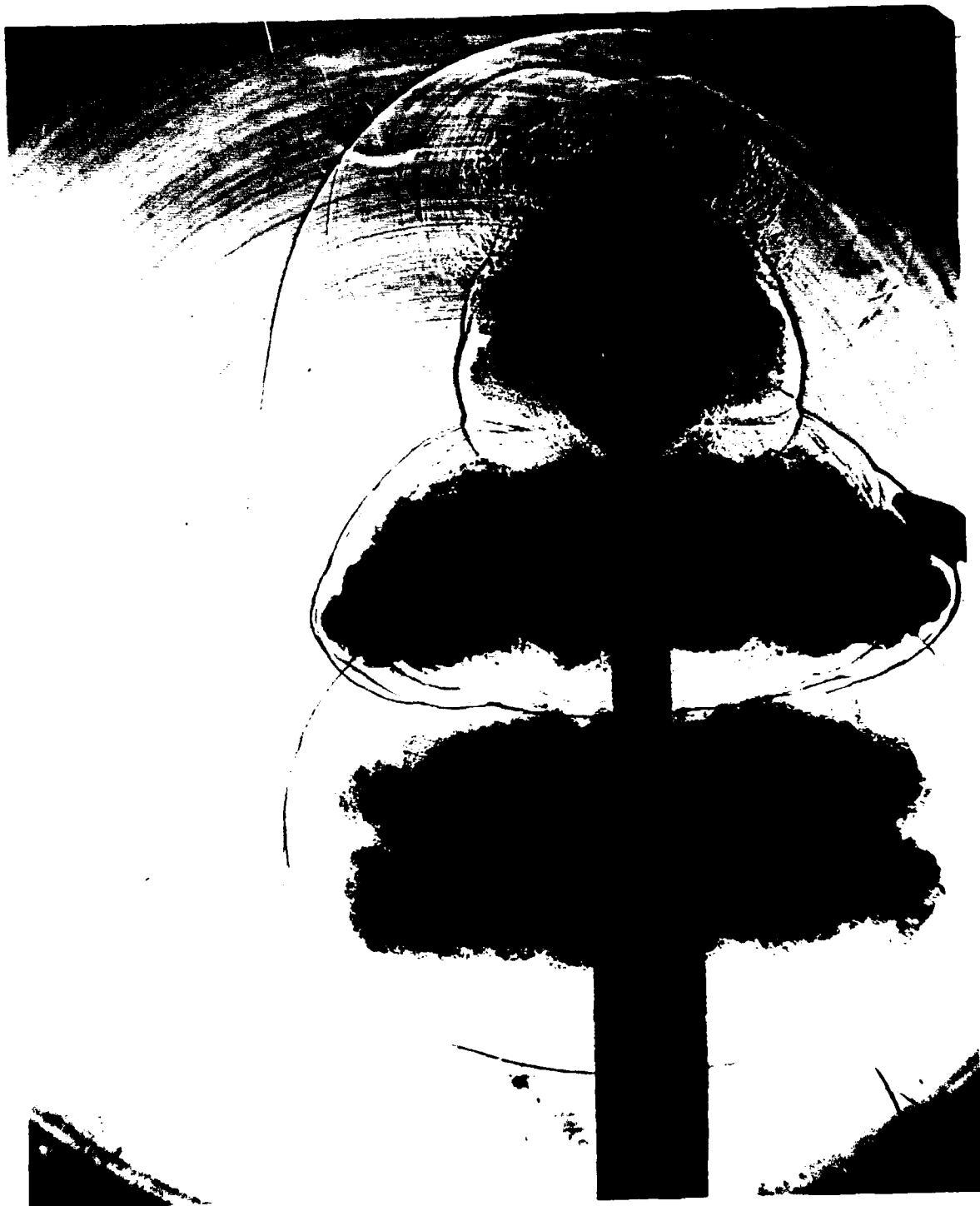
Figure B9b. Shadowgraph for round 19550, split brake, taken with a 150-microsecond time delay.
