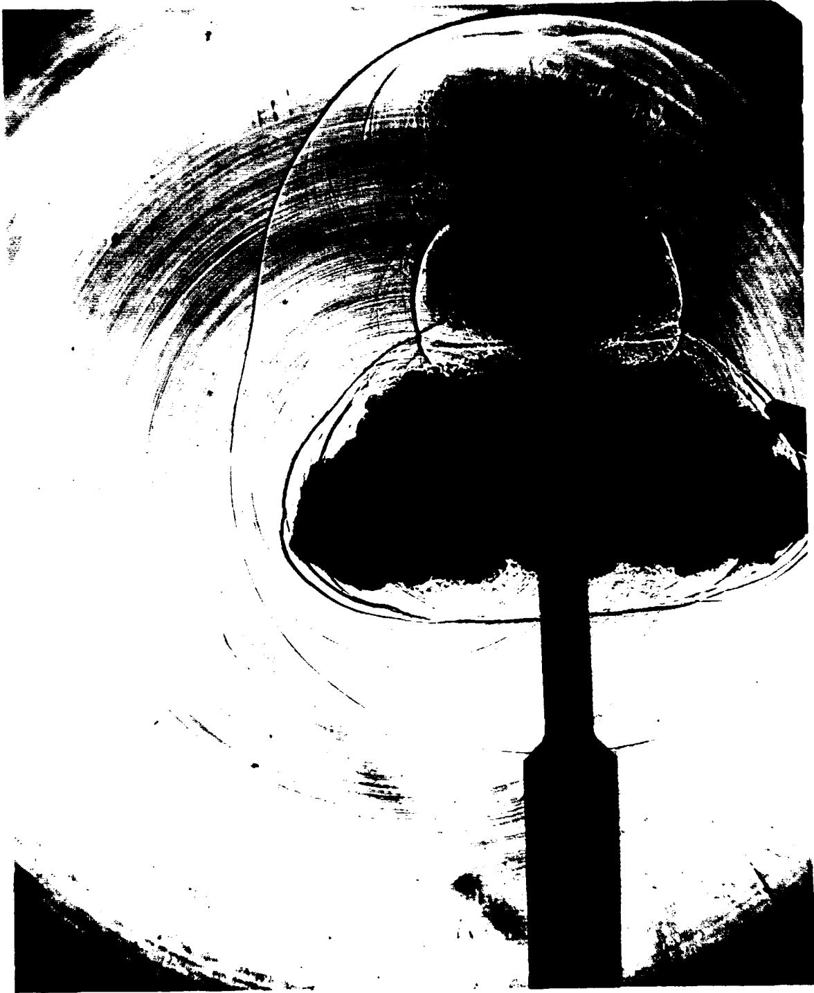
Figure B6b. Shadowgraph for round 19544, standard brake, taken with a 150-microsecond time delay.
