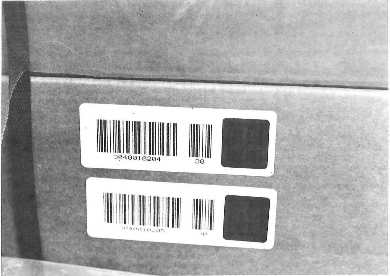
Figure 17. Time-Temperature Indicator Labels on Outside of Ration Cartons.
