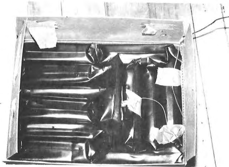
Figure 14. Open Case of MRE Rations with Thermocouples Attached
