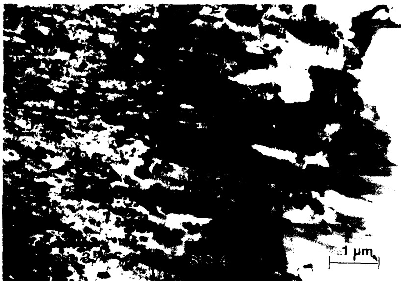
Fig. 5. TEM micrograph of the SiC-3/SiC-4 interface. The SiC-3 region and the inner ( \sim 3 \mu\text{m} ) part of the SiC-4 region are very similar to the same regions in the as-received fiber, except for the carbon segregation to the junctions of the SiC grains in the SiC-3 layer. The grains in the outer parts of SiC-4 are greatly coarsened.
