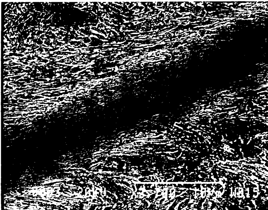
Figure 10. Further enlargement of Figure 7 showing details of the shear band.
