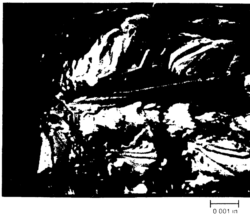
Figure 23. Fatigue crack initiation in open hole specimens from constituent particles in thin plate. (a) Constituent particle size = 0.00097 in. and (b) constituent particle size = 0.0009 in
