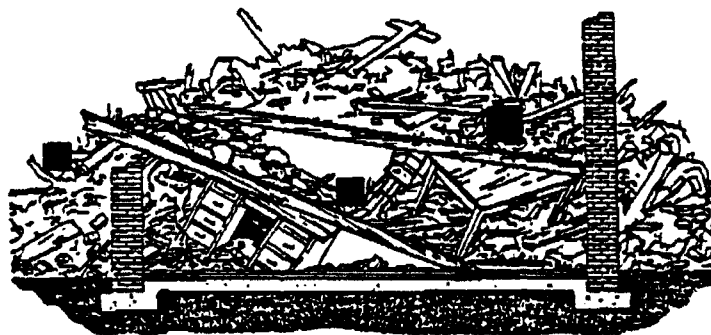
Pancake floor collapse
