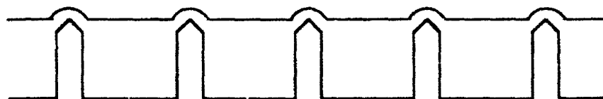
Step 3: Deposit oxide layer
