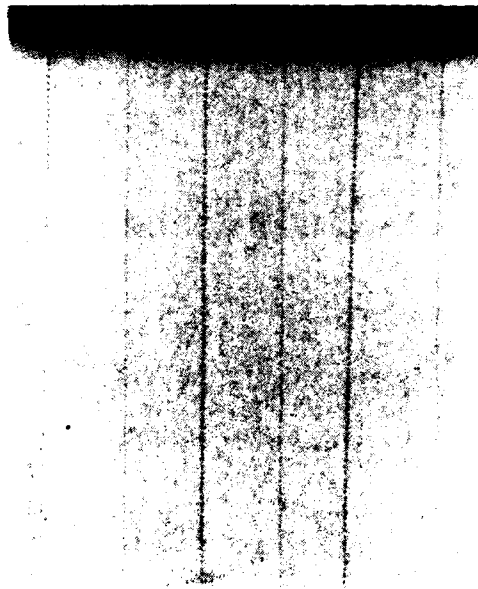
Figure 20. A Jet Array of Alternating 8 and 18 Micron Diameter Jets, is Acoustically Driven at 220 kHz
