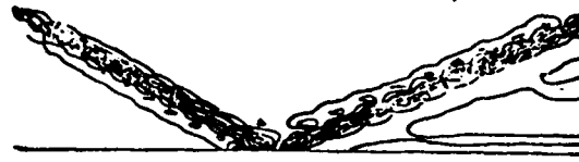
Fig. 4. Equal-Mach-number curves for shock reflection at solid wall M_{\infty} = 2.9 , \Delta M = 0.0666
