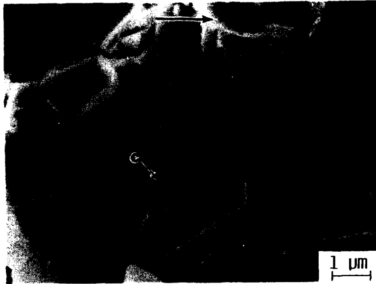
Fig. 4.16. SEM micrograph of a Nb particle in the equiaxed Nb/Nb 3 Al composite under cyclic loading at 25 Hz and room temperature, showing evidence of "cyclic cleavage". Note the presence of striations perpendicular to the crack-growth direction (direction of arrow) and also perpendicular to the cleavage river markings.
