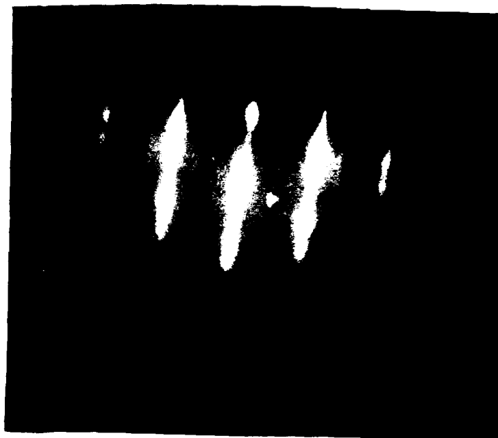
Figure 2. RHEED image of a \beta -SiC layer ([110] azimuth) grown on off-axis \alpha(6H) -SiC.
