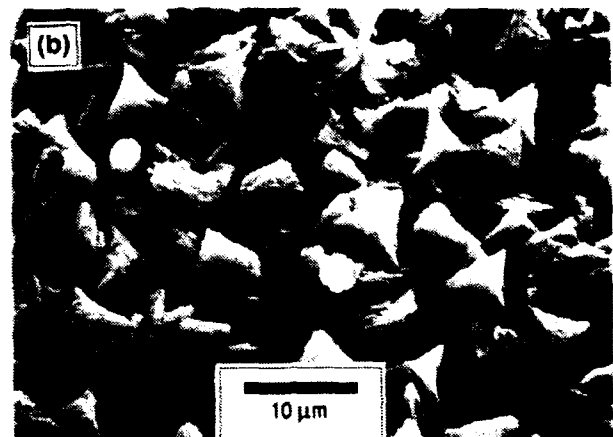
FIGURE 2 – Calcareous deposits on polarized 304 stainless steel after 43 days
