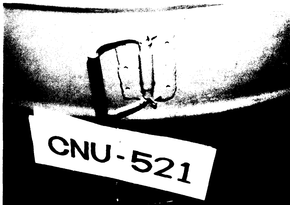
Figure 50. Hoisting Fitting Strength Test, CNU-521/E Drum, Horizontal Carriage Handle Deformation.
