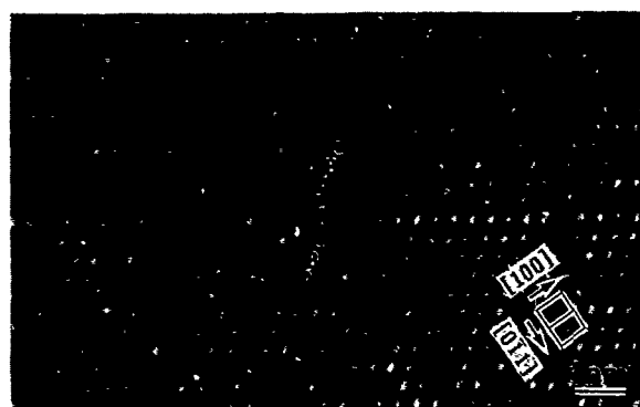
Fig. 6. A high resolution electron micrograph of a \{111\} stacking fault.
