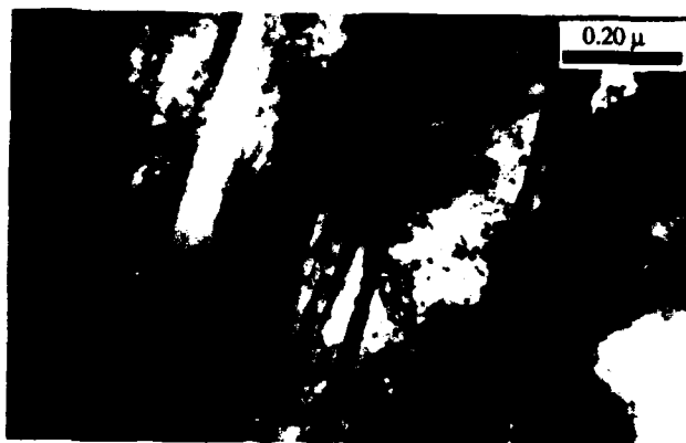
Fig. 5 (a) Microtwin substructure formed after 0.46 \epsilon_c TMT at 454°C. Bright field image.
