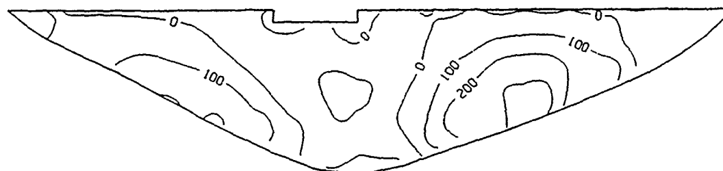
D/S CANTILEVER STRESSES
