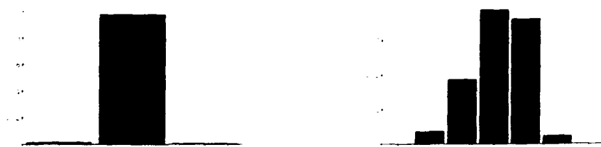
Figure 4.2: Distribution of Delay Cycles for N_s = 4 and 16, respectively Using B_{192} Leaves.
