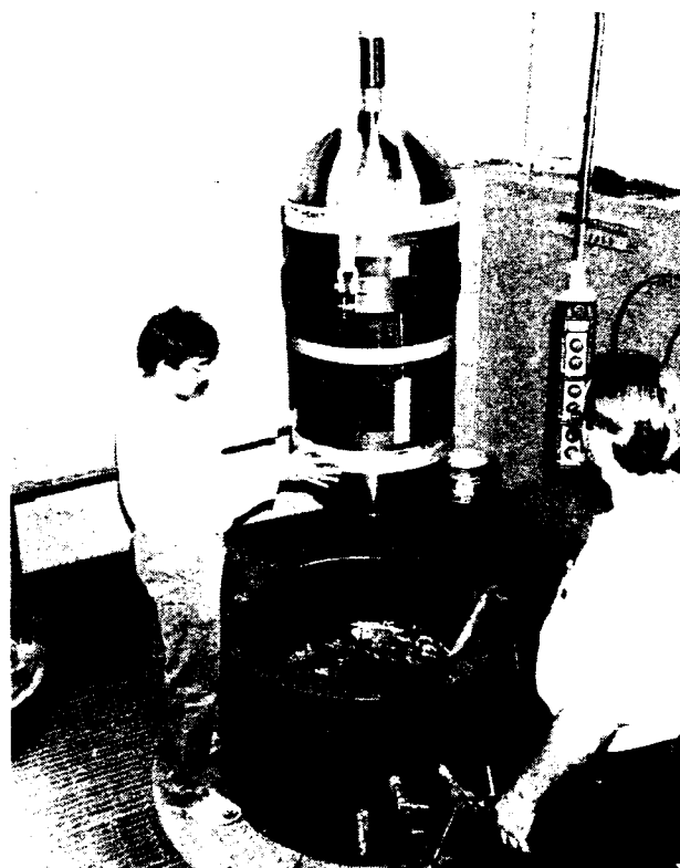
Figure 35. Placement of the 20-inch OD ceramic housing test assembly into the 30-inch ID pressure vessel at the Southwest Research Institute.
