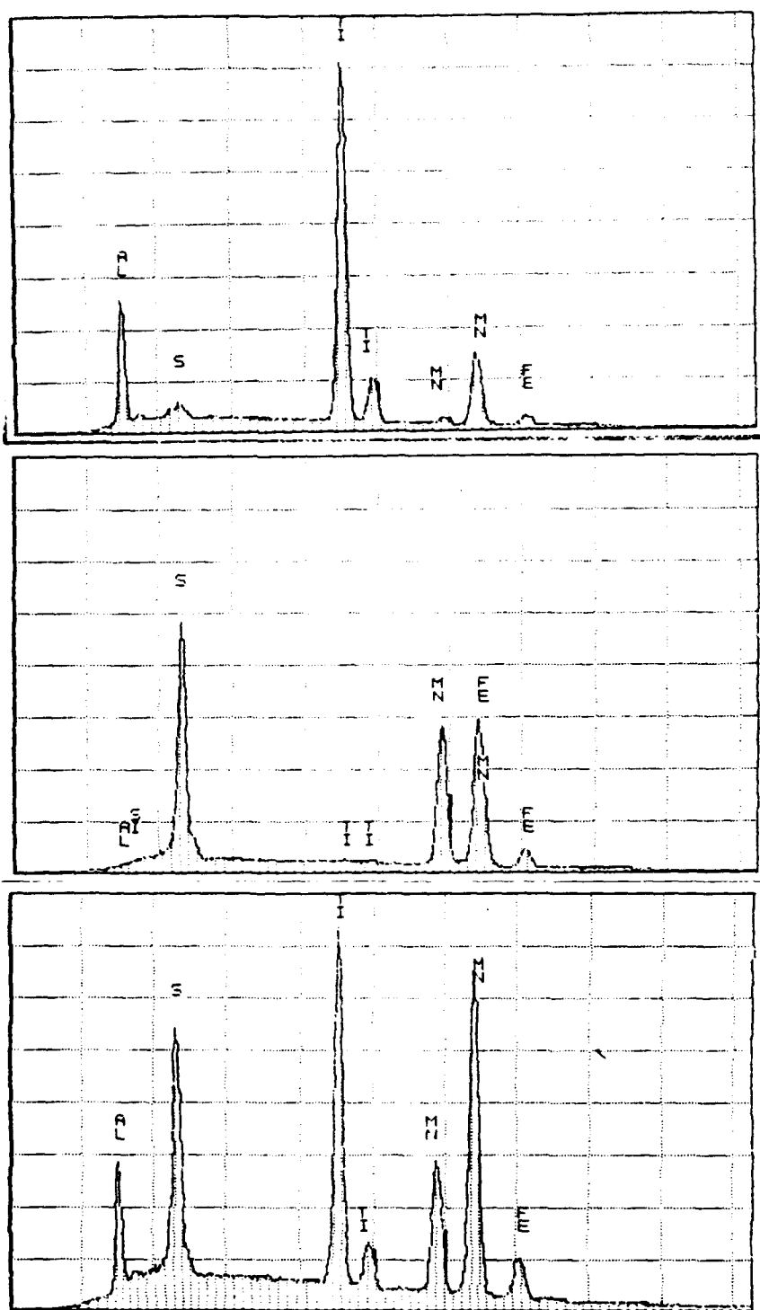
Figure 3.2 Representative of EDS spectra for inclusions in steels A, B and C.
