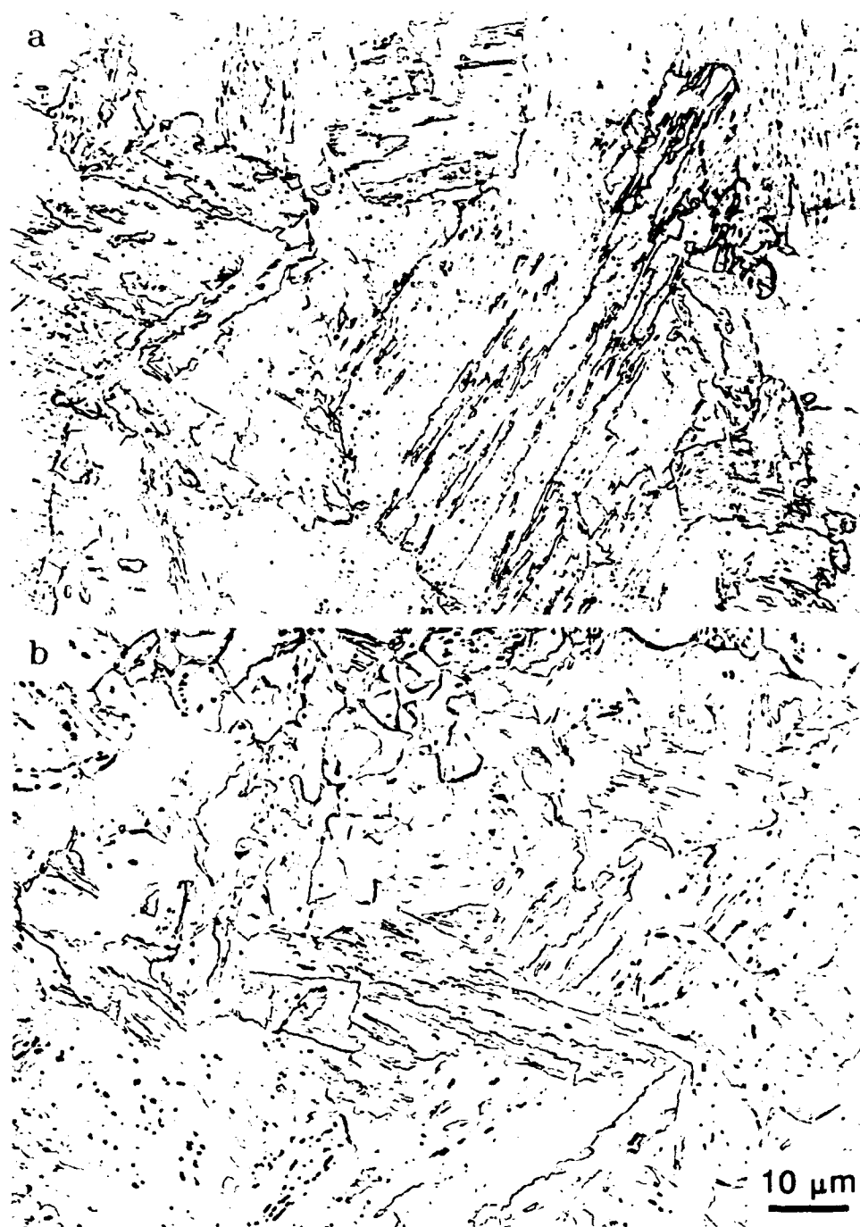
Figure 3.16 Martensitic microstructures in specimens cooled at 150°C/s. (a) 1X condition and (b) 2X condition. Light micrographs.
