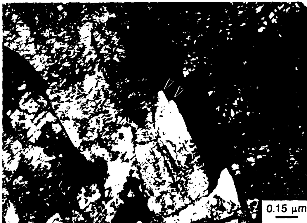
Figure 3.31 The edges of "bainitic" ferrite subunits. Specimen cooled at 3.3°C/s, 1X condition.
