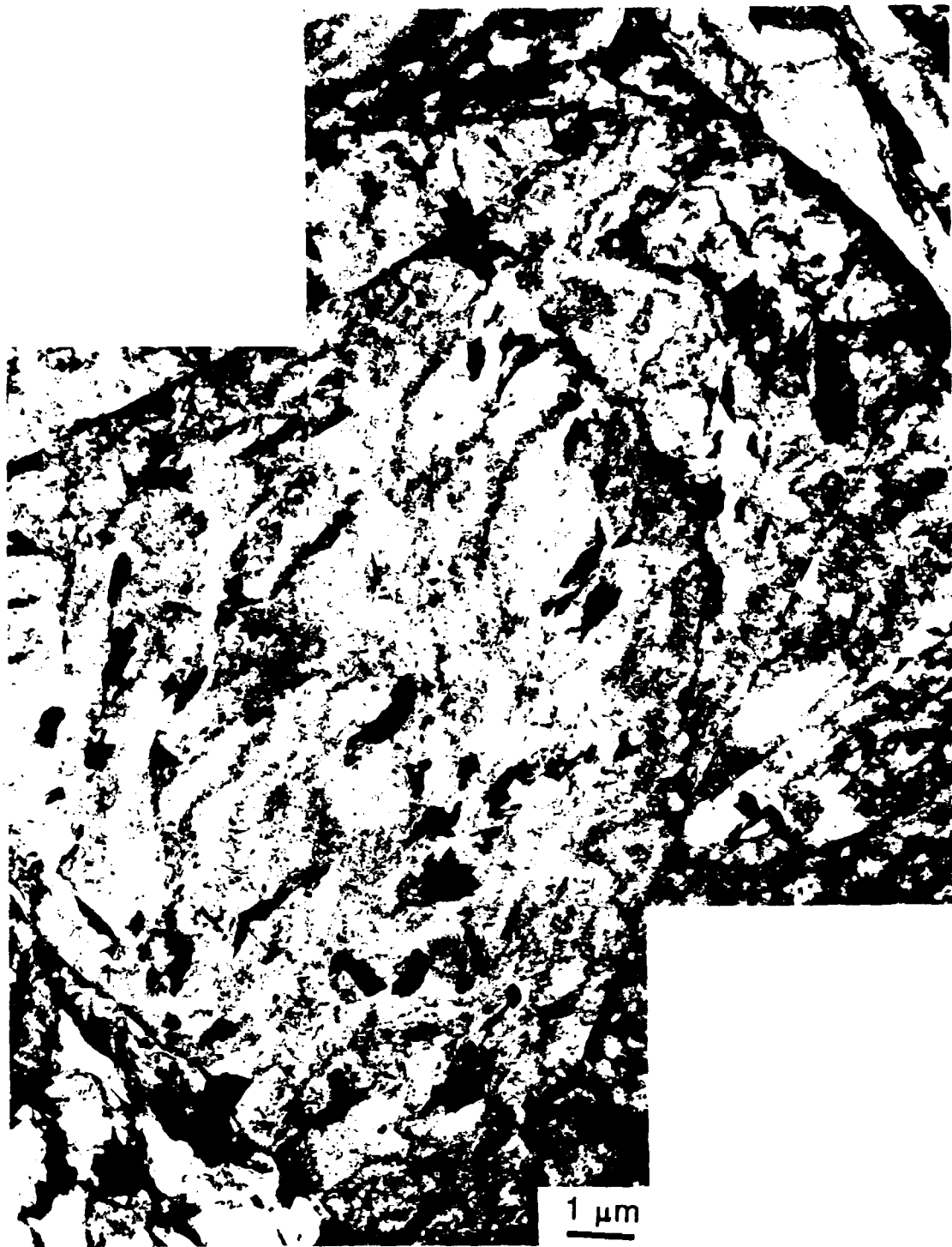
Figure 3.14 Microstructure of the as-received steel B. Notice the black M-A islands.
