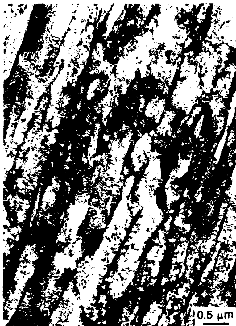
Figure 3.22 Microstructure of specimen cooled at 25°C/s for the 1X condition.
