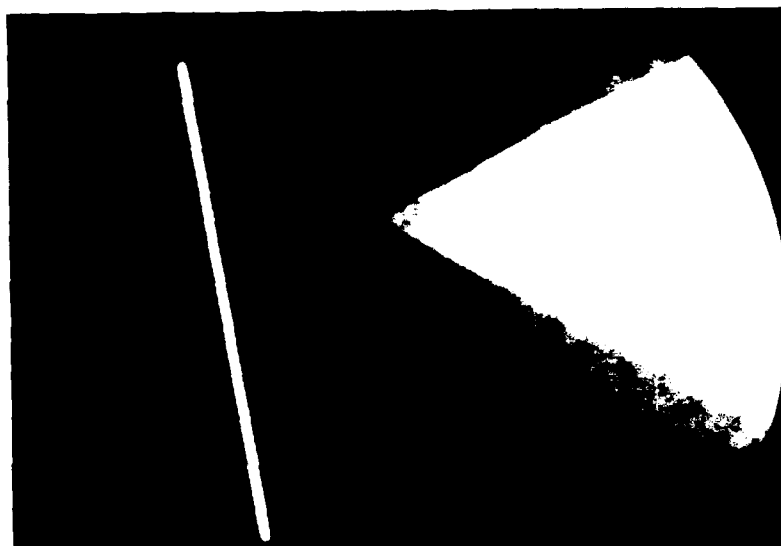
Figure 3.3.1-4 CT image of "V" section for article 2.
