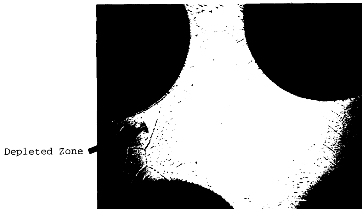
Figure 4.5 Heat Treated Microstructure SCS-6/Ti-15-3 (500X)
