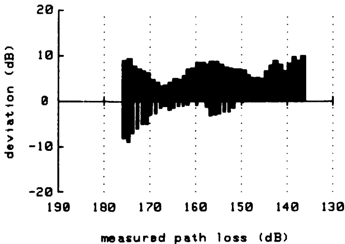
fig. 18d Comparison between the measured and predicted 16 GHz path losses of the Lorient period.
