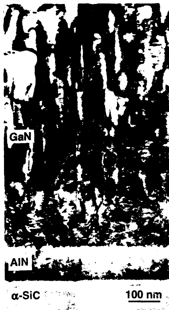
Figure 8. TEM micrograph of GaN(650°C)/AlN(1100°C)/α-SiC, the deposition rate for the GaN film was five time less than the rate for the GaN film in Figure 6.
