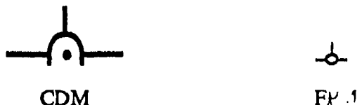
Figure 4. The CDM and FPM symbols used in the standard HUD symbology set.
