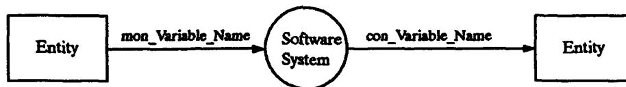
Figure 5-7. Representation of an Overview of a Specification Using a Context Diagram
