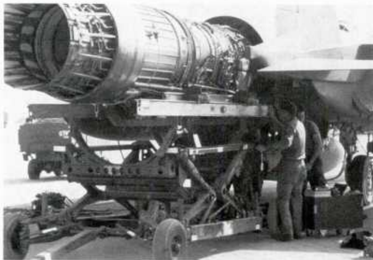
Figure 21. Removing an F-15 Engine. The present maintenance concept allows for a jet engine intermediate maintenance capability within the 366th Wing for the F-15C/E and F-16C aircraft. KC-135 engine maintenance will remain as an off-base maintenance capability.
